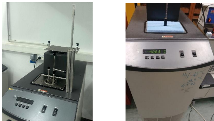
Figure 5. Bath for realizing the mercury triple point with the mercury cell
