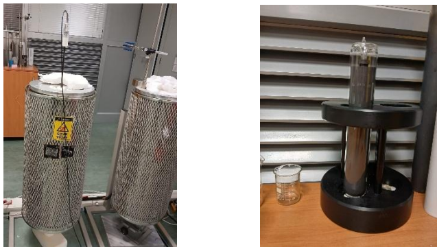
Figure 2. Tin fixed-point cell in furnace with SPRT (left) and the tin fixed-point cell (right).
