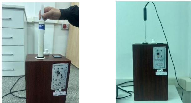
Figure 3. Gallium fixed-point cell in a heated isothermal enclosure
